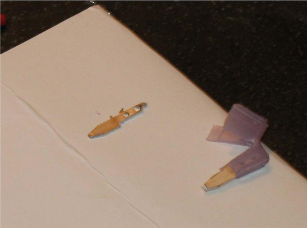
Once you have a good connection, heat-shrink the area that would normally be covered by the fuse housing.
