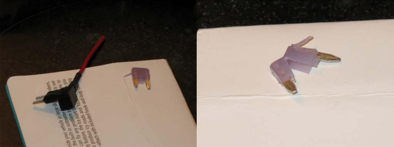
Cut the fuse open, holding one fuse blade in the needle nose pliers, cut the plastic off with the wire cutters.
